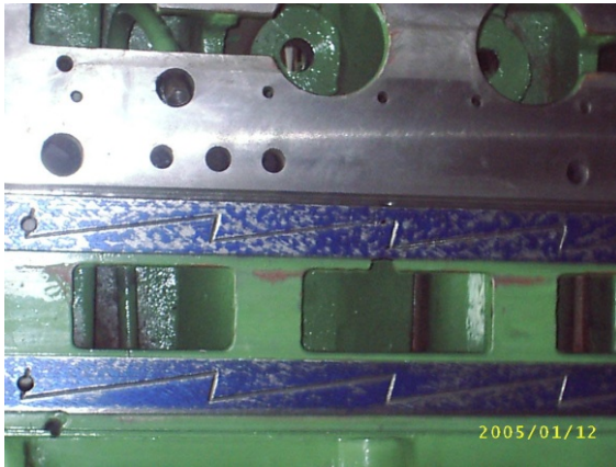
Fig. 8. Guides with lubrication channels in the manual processing phase.
