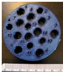
Fig. 2. Specimen with counterbore vertical axes holes (specimen 9).
