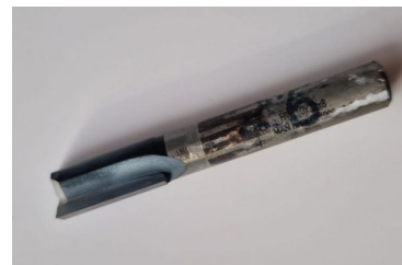
Fig. 1. Two flutes end mill of 10 mm diameter.
