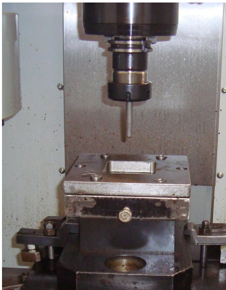
Fig. 5. Tool system fixed on HAAS MiniMILL milling center.
