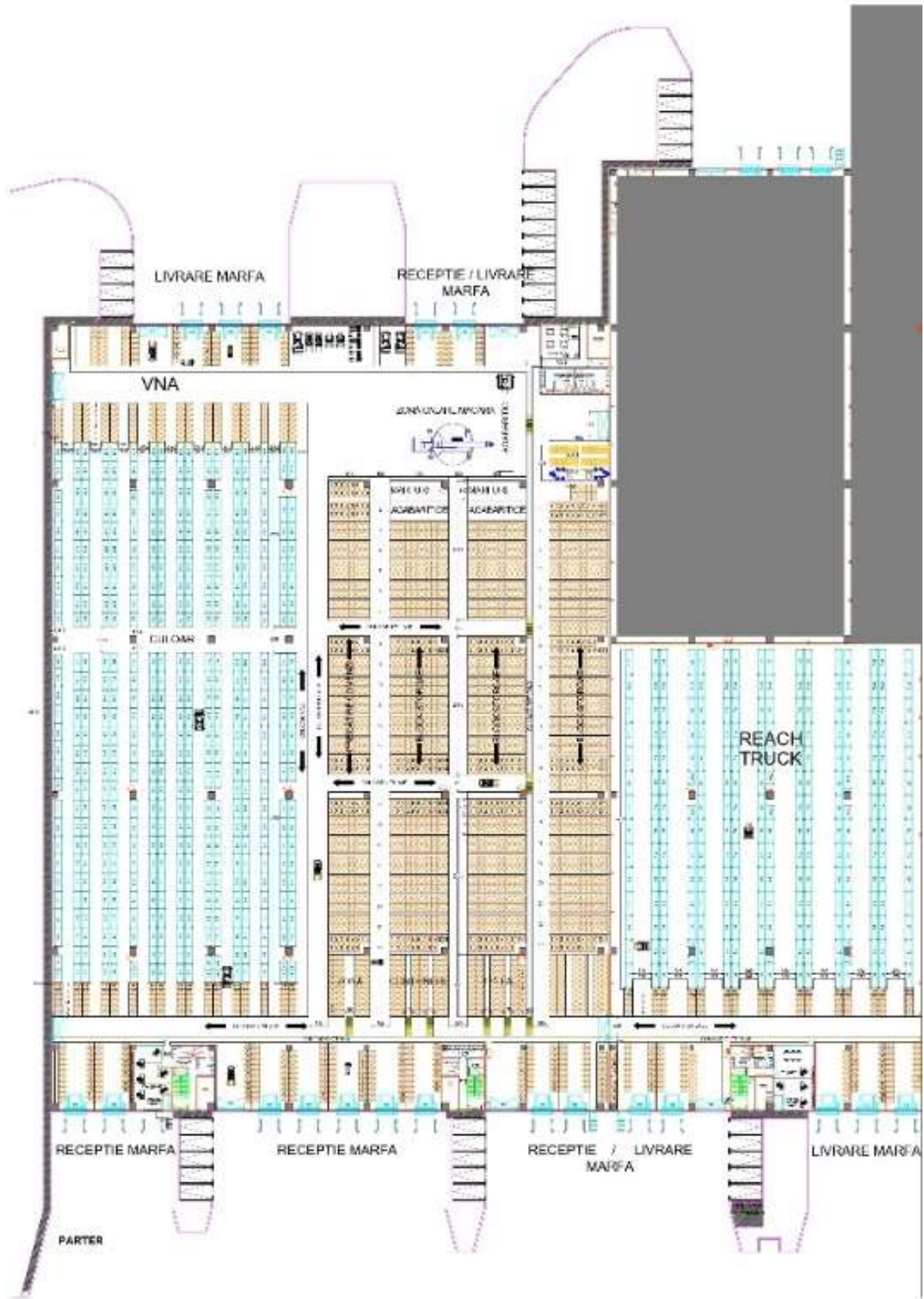
Fig. 1. Warehouse layout subject of data simulation.
