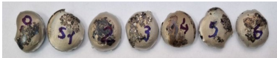
Fig. 3. Samples of experimental biocompatible stainless steels doped in different proportions with Cu, Ag and Ti.
