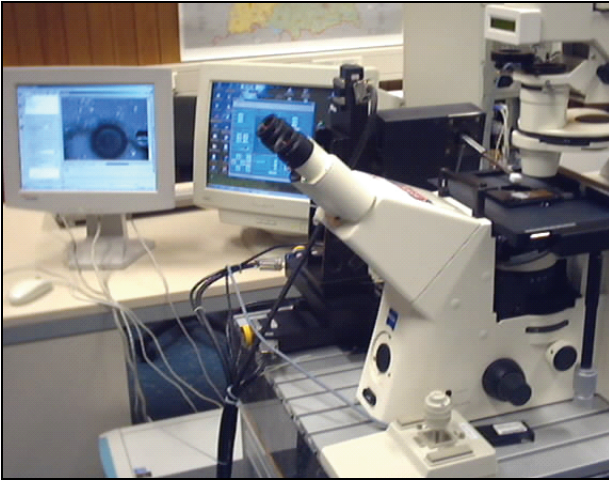
Fig. 1. General View of the robot system equipped with Microscope Carl Zeiss Axiovert 200.
