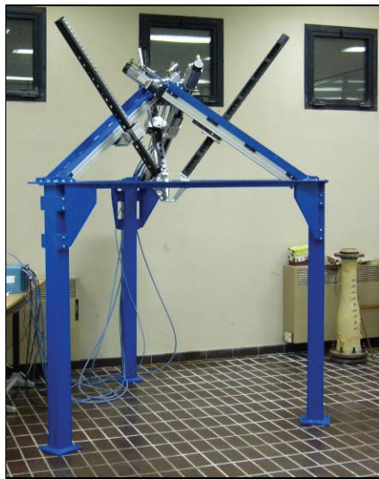
Fig. 7. Architecture of the assembly system based on cooperating parallel robots.
