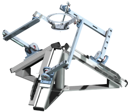
Fig. 8. Prototype of translation robot (a) and final design of spherical wrist (b).
