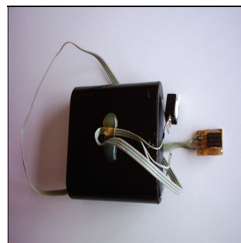
Fig. 6. The ADXL 190 WQC acceleration sensor and the available supply source.
