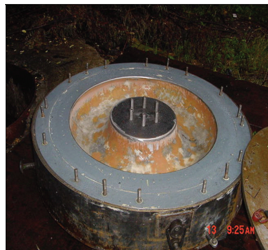
Fig. 3. Die ready for underwater explosion.
