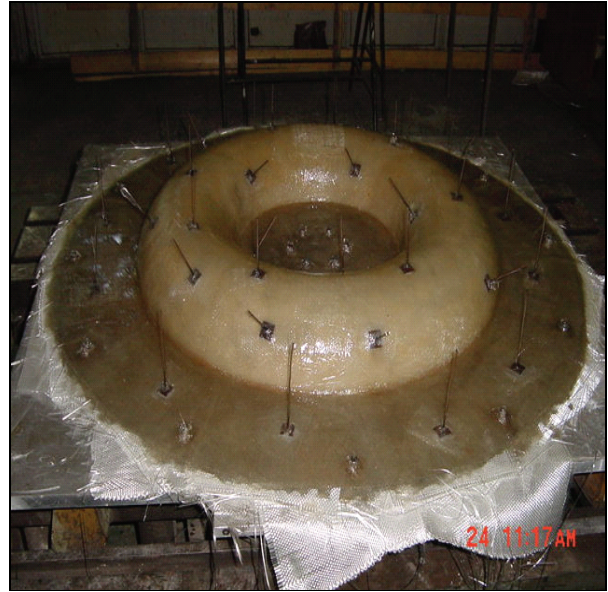
Fig. 1. The master coated with epoxy resin reinforced with fiber-glass.
