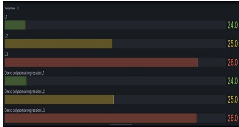
Fig. 5. Comparison between temperature setpoints and measured temperatures for the three cooling loops, including polynomial regression trends used as Digital Twin estimates of the thermal behavior.
