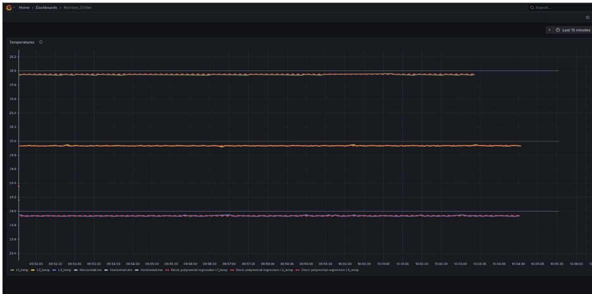
Fig. 4. Grafana dashboard showing polynomial regression–based stability analysis of the three Mydax chiller cooling loops, including measured temperatures, setpoints and regression trends used for long-term stability evaluation.
