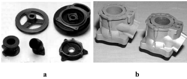
Fig. 5. Pieces obtained: a - in shapes made through rapid procedures [15]; b - through DSPC procedure [18].
