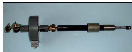
Fig.2. Magnetorheological damper with inductive transducer.
