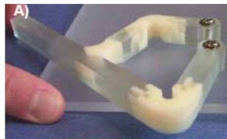
Fig. 7. Prototype with insertion manufactured using RP.
