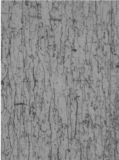
Fig. 5. Initial microstructure for the sheet g = 0.5 mm ( \times 125 ).
