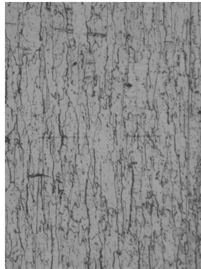
Fig. 12. Deformed microstructure in the area of the fillet radius, for the case g = 1 mm, D_p = 16 mm and h = 6 mm ( \times 125 ).
