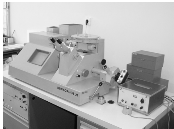
Fig. 4. The Neophot 21 microscope used for the micro structural analyses.
