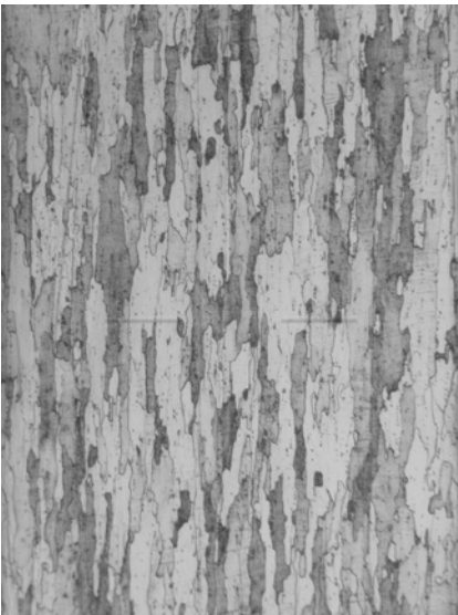
Fig. 9. Deformed microstructure in the area of the part bottom, for the case g = 0.5 mm, D_p = 20 mm and h = 6 mm ( \times 125 ).
