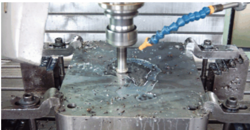
Fig. 2. Rough milling of movable die insert shape.
