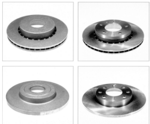
Fig. 2. Casts and final shape of brake discs [1].
