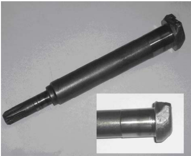
Fig. 3. Defects that appear on the eccentric shaft.
