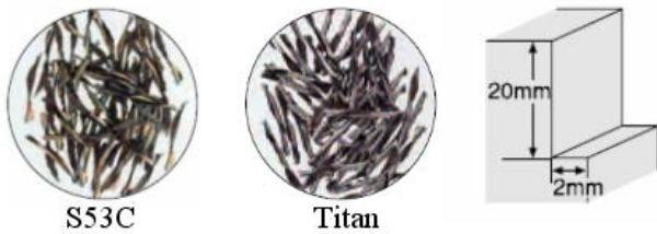
Fig. 14. Types of swarf depending of the material.
