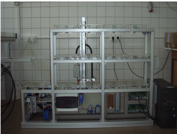
Fig. 6. Shelf storage manipulator in real.
