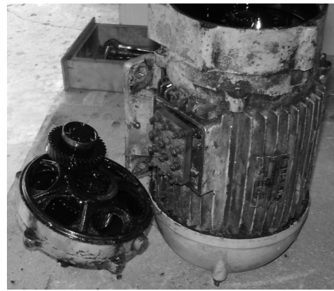
Fig. 9. Reducer and electric motor.
