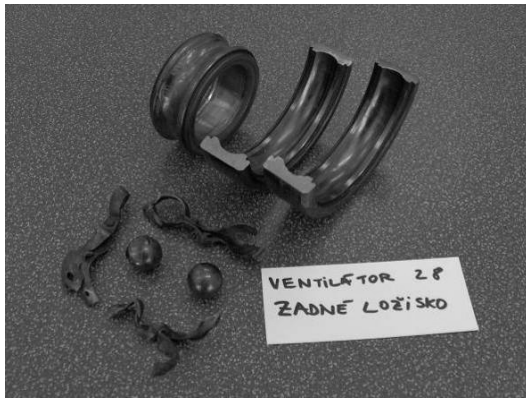
Fig. 14. Damaged tail bearing.
