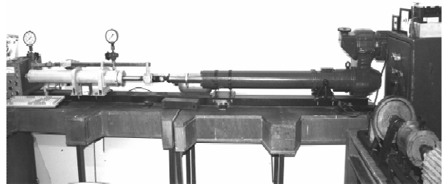
Fig. 8. The test stand for linear electro-mechanic actuator.
