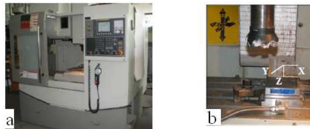
Fig. 1. MCV 300 machine-tool: a – basic components; b – machine-tools dynamometer axis system.
