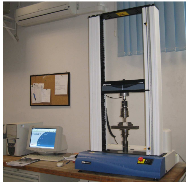
Fig. 2. Test bench used in the three-point bending tests.
