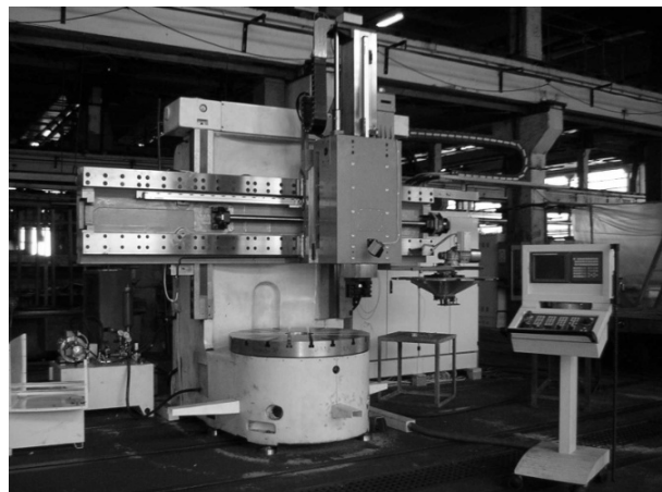
Fig. 5. Vertical lathe with 2-speed gearbox with toothed belt, without pinion/crown mechanism.
