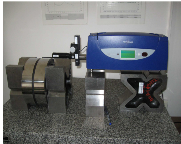
Fig. 2. Roughness measuring device Taylor Hobson.
