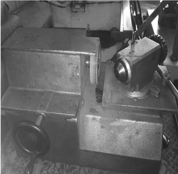
Fig. 10. Device for grinding valves.
