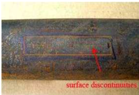
Fig. 3. Starting material – surface discontinuities.
