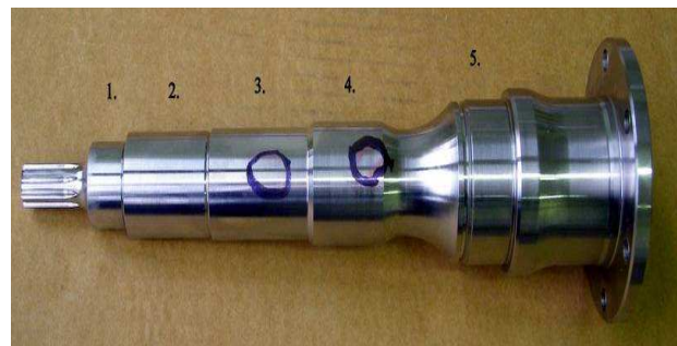
Fig. 2. Damage to the shaft before further processing and hardness measurement points (1–5).
